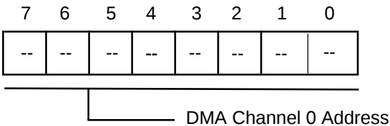
Figure 55. DMA Source Address Register 0L
