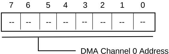
Figure 56. DMA Source Address Register 0H
