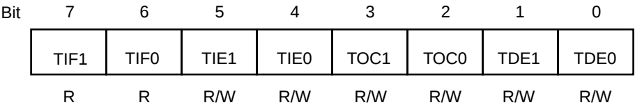
Figure 46. Timer Control Register (TCR: I/O Address = 10H)
