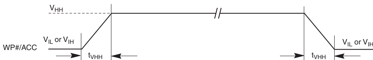
Figure 17.12 Accelerated Program Timing Diagram
