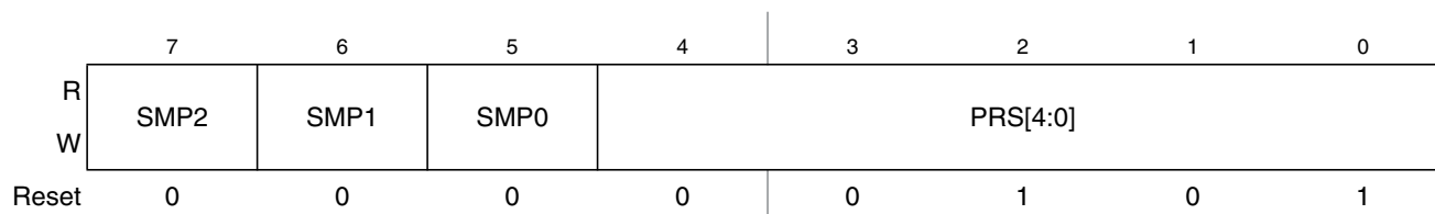
Figure 15-7. ATD Control Register 4 (ATDCTL4)
