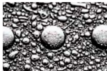
MT Connector Cleaned with IPA
