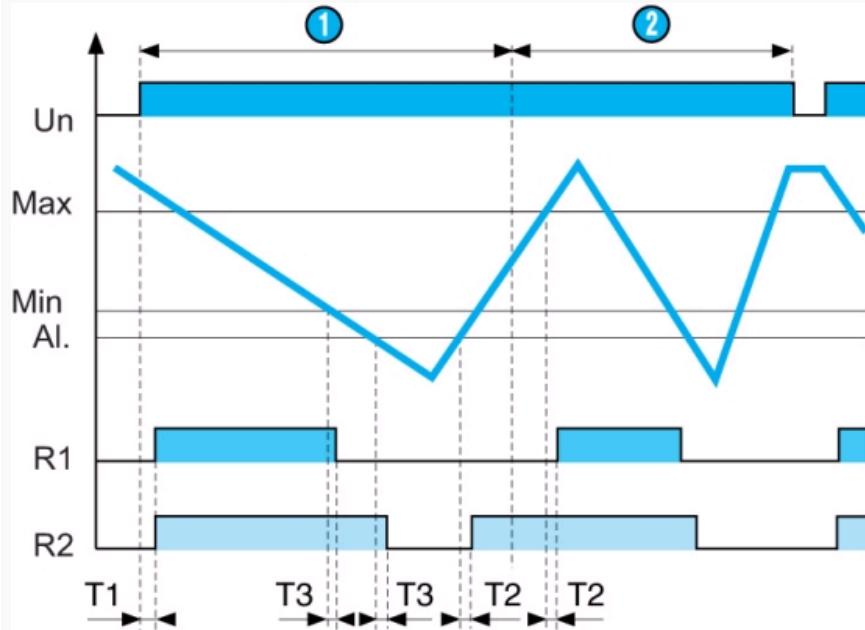
On power-up, probes Min, Max and Al. are submerged, relays R1 and R2 are energised and the pump is ON : emptying starts, the LED for relay R1 is lit. When the Min probe emerges, relay R1 goes off. If, in the event of a fault, the level continues to fall and probe Al. emerges, relay R2 de-energises and the alarm is triggered : the LED relay R2 is lit. This fault can be stored.
