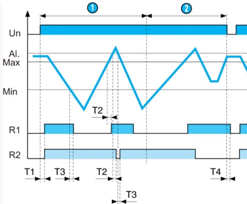
On power-up, probes Min, Max are submerged and probe Al. is above the level of the liquid. Relays R1 and R2 are energised and the pump is ON : emptying starts, the LED for relay R1 is lit. When the Min probe emerges, relay R1 de-energises and the pump if OFF : emptying stops, the LED for relay R1 goes off. If, in the event of a fault, the level continues to rise and reaches probe Al., relay R2 de-energises and the alarm is triggered : the LED for relay R2 is lit.
