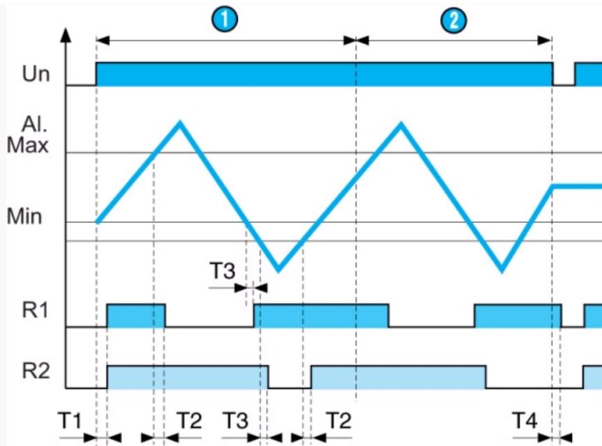
On power-up, probe Al. is submerged, relays R1 and R2 are energised and the pump is ON : filling starts, the LED for relay R1 is lit. When the level reaches the Max probe, relay R1 de-energises and the pump is OFF : filling stops, the LED for relay R1 goes off. Relay R1 re-energises when the Min probe emerges. In the event of a fault (level continues to fall) probe Al. emerges, relay R2 de-energises and the alarm is triggered : the LED for relay R2 is lit.
