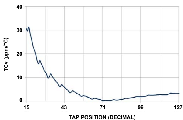
FIGURE 14. 50kΩ TCv vs TAP POSITION, V_{CC} = 3.3V
