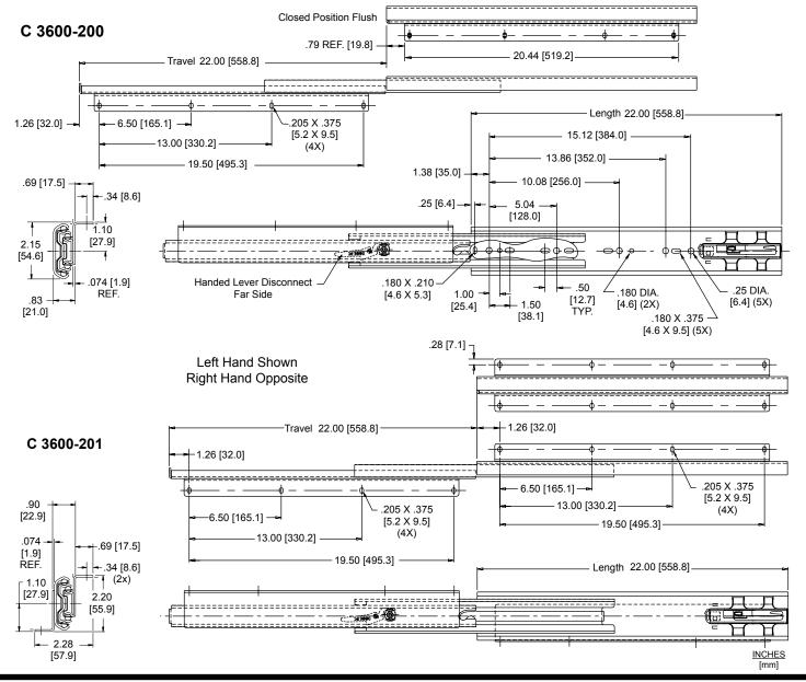
Finishes Bright electro-zinc (C) plating only Mounting 3600-200: Fixed inboard bracket
