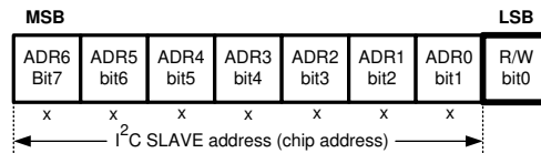
Figure 16. I 2 C Chip Address (0x2C)
