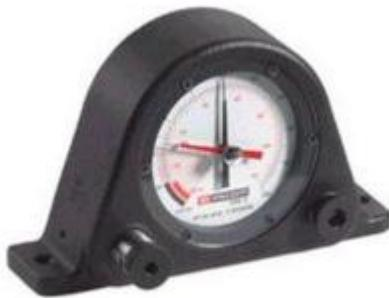
Screwdriver torque-meter CDS.2 by Facom, with capacity 10-70 Nm. Accuracy :  $\pm 2\%$  from 20 % to 100 % of full scale reading. Numbered and supplied with a calibration certificate. Large-diameter dial with reference pointer for clear, error-free readings. Complete with 2 square drives. Tool, manufactured by Facom.
