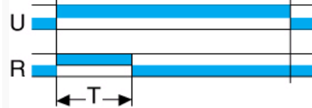
Function H - 1 relay output
