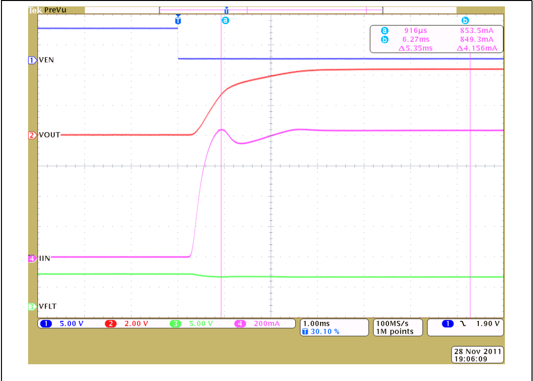
Figure 17. Soft-start performance for 100 \mu F capacitive load
