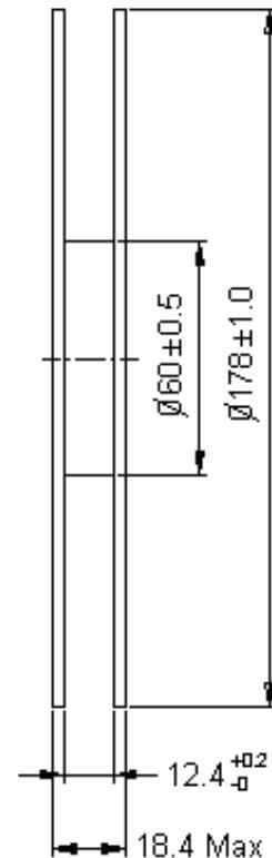
Note: 01. The tolerance unless mentioned is  $\pm 0.1$  mm
