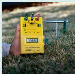
Check resistance between earth and grounding rod.
