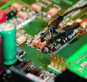
Our alligator and crocodile clips have the right bite size for every occasion: sheets, bolts and automobile batteries, use in acceptance inspections in industrial manufacture or even for electrical supply to electrochemical accessories. They are used wherever variable clamping with low contact resistance is required. Their powerful teeth and the gentle fine wire clamping area make them the universal and high-stress bearing tool for the measurement and transmission of currents.
