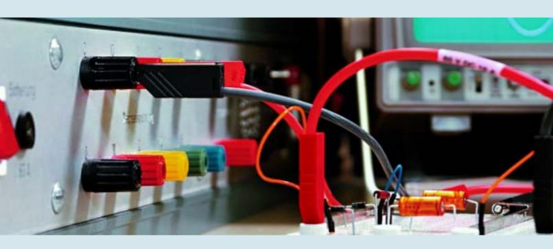
You can fit them quickly, and thanks to their long life, forget them as well: Hirschmann sockets and couplings provide quick and uncomplicated connections of measuring leads and plugs in devices, covers or panels and can be used for setting up circuits, for example. In the pole clamp version, they can be used for sub-clamping of leads and cable lugs in practice.
