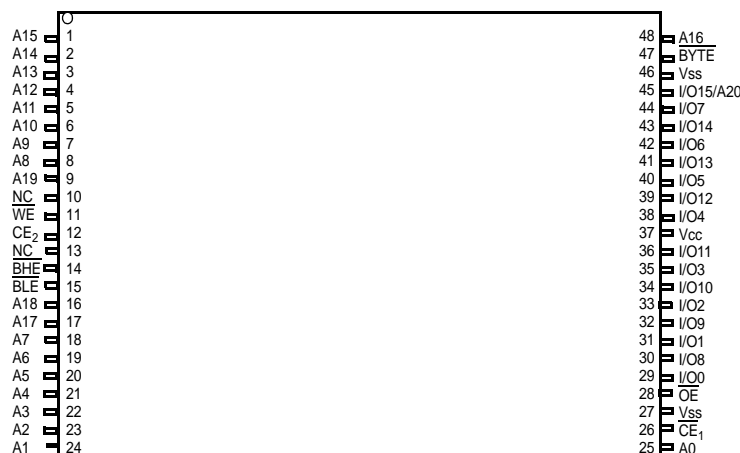
Figure 2. 48-pin TSOP I pinout (Top View) [2, 3]
