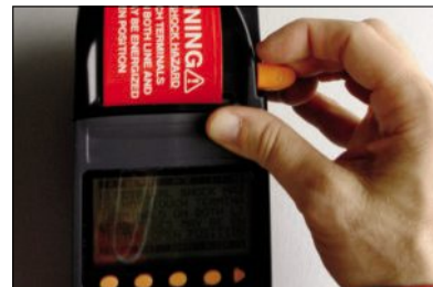
Step 3) Remove and apply your printed label.
