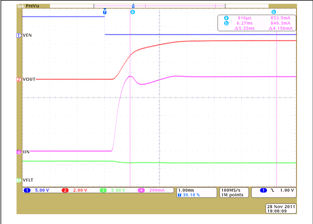
Figure 17. Soft-start performance for 100 \mu F capacitive load
