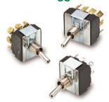
General purpose workhorses with options tailored to meet UL/CSA: 1000V-live to dead metal most any need. Ratings to 17A 125VAC, various actuator, bushing, termination, and circuit choices allow this toggle to easily integrate into a variety of different applica- 50,000 cycles- maintained tions. The H/I-Series has a storied history in the Food service, Generator, Industrial Control, and Office Automation markets and are appropriate for usage in low voltage DC applications as well.
