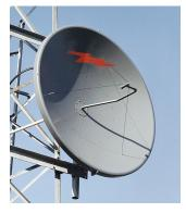
3.7 m | 12 ft Standard Parabolic, Low VSWR Unshielded Antenna, dual-polarized, 7.125–8.500 GHz, CPR137G, gray antenna, with flash, standard pack—two-piece reflector
