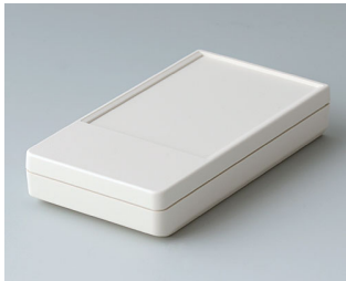
A9070107 DATEC-POCKET-BOX S ABS (UL 94 HB) off-white RAL 9002 3.35"x1.81"x0.63" IP 41
