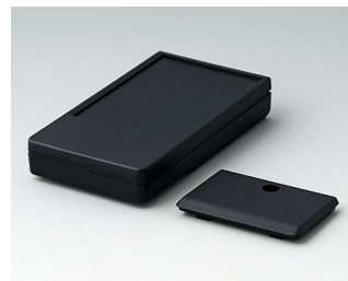
A9071109 DATEC-POCKET-BOX M ABS (UL 94 HB) black RAL 9005 4.13"x2.28"x0.73" IP 41
