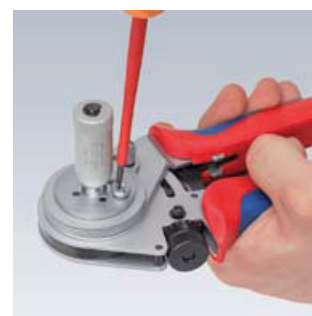
Locator 97 59 65 2 for four-mandrel crimping pliers, adjustable in length and diameter for various plugs
