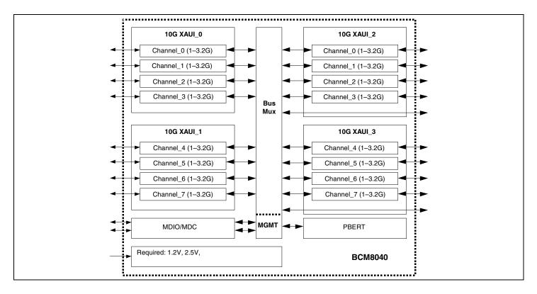
The BCM8040 device integrates 4 independent XGXS (XGMII eXtender Sublayer) cores leveraging Broadcom's high-performance mixed-signal design experience along with advanced 0.13-μ CMOS process technology. Combine this with a robust architecture offering the highest degree of flexibility and the result is a highly programmable, lowest power retimer solution for network line card and backplane applications.
