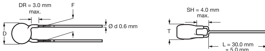
Capacitors with 5.0 mm, 7.5 mm and 10 mm lead spacing
