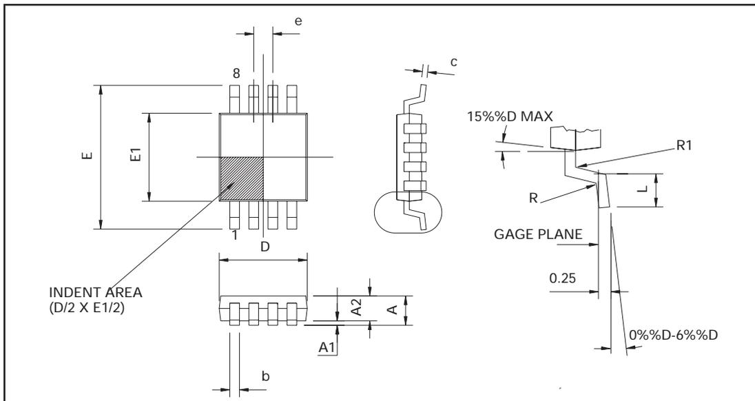
Controlling dimensions are in millimeters. Approximate conversions are given in inches
