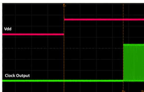
Figure 17. Startup Waveform vs. Vdd
