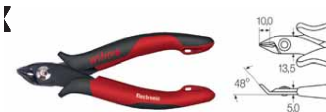
wide, pointed head without bevelled edge
