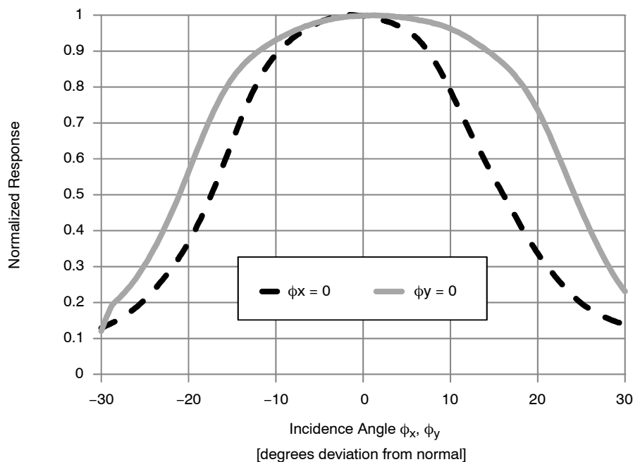
Figure 5. Central Pixel Photoresponse to a Fixed Optical Power with Incidence Angle varied along \phi_x and \phi_y
