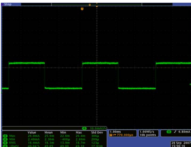
FIGURE 12. I_{LED} AT 50% PWM DIMMING (54 LEDs, 20mA, V_{IN} = 12V )
