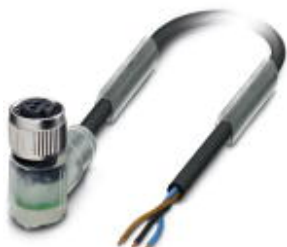
Sensor/actuator cable, 3-position, PUR halogen-free, black-gray RAL 7021, free cable end, on Socket angled M12 SPEEDCON, A-coded, with 2 LEDs, cable length: 10 m
