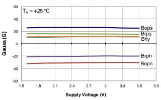
Switch Points vs Supply Voltage
