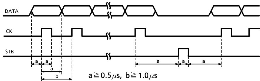
The data to the DATA terminal is input to the internal shift registers sequentially with synchronizing to the rise of the input to the CK terminal.
