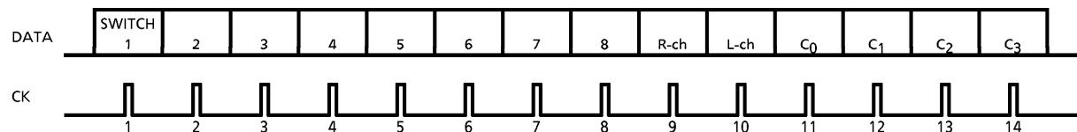
As the bit 1~8 correspond to the analog switches 1 to 8 respectively, set the bit of the desired switch to the level "1" (see Note).
