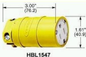
2-Pole 3Wire Grounding, 15A 125V, 150R, Yellow Elastomer, Dust Tight
