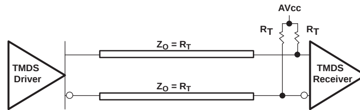
Figure 1. Termination for TMD5 Output Driver
