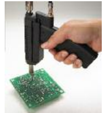
Through hole desoldering with the MX-DS1 hand-piece.
