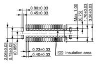
Recommended metal mask pattern Metal mask thickness: When 150μm (Terminal opening ratio: 48%) (Metal-part opening ratio: 100%)
