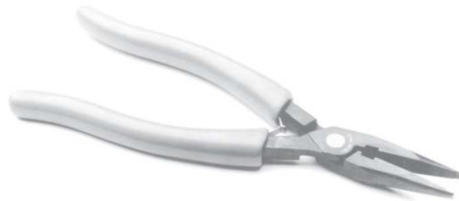
The jaw tips are shaped to grip a right angle MCX plug body for insertion or disengagement to a mating receptacle. The jaws are hardened steel and the handles are cushioned to minimize stress to the user. For use with all cable groups except RG-58.
