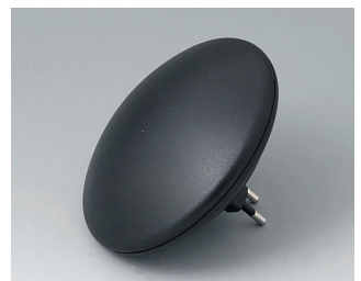
B5011129 ART-CASE R110 H PC+ABS (UL 94 V-0) black RAL 9005 ø4.33"x1.50" IP 40
