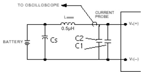
$L_{test} = 500nH$     $C_s = 270\mu F$     $Esr < 0.1 \text{ ohm at } 100\text{kHz } 20^\circ C$
