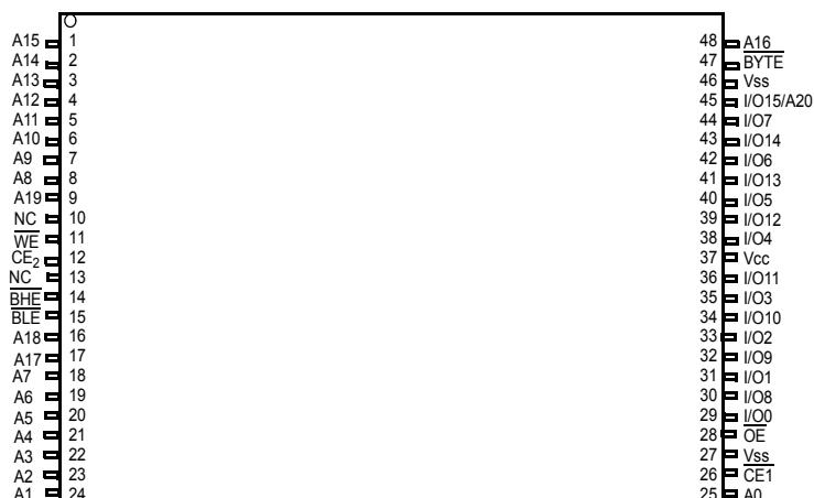
48-pin TSOP I pinout (Top View) [1, 2]
