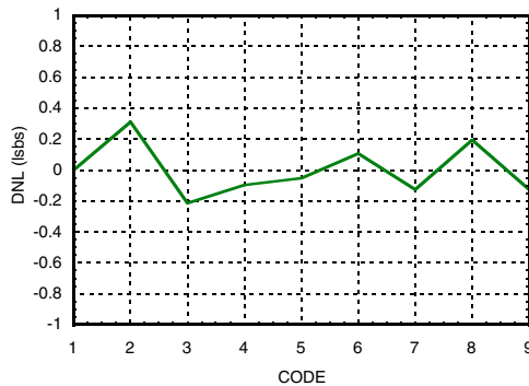
Differential Nonlinearity (Including overrange bits)
