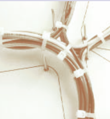
Wire and Cable Bundling (Harnessing)
