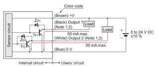
Notes: 1) Make sure to connect terminals correctly as the sensor does not incorporate a reverse polarity protection circuit.
