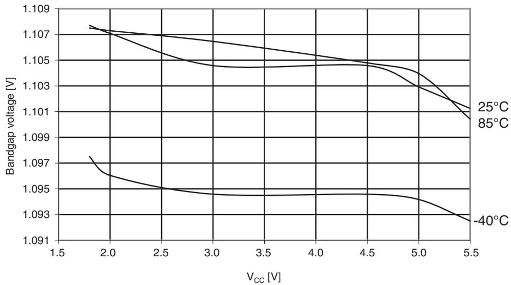
**Figure 30-84. ATmega164PA: Bandgap voltage vs. temperature**
