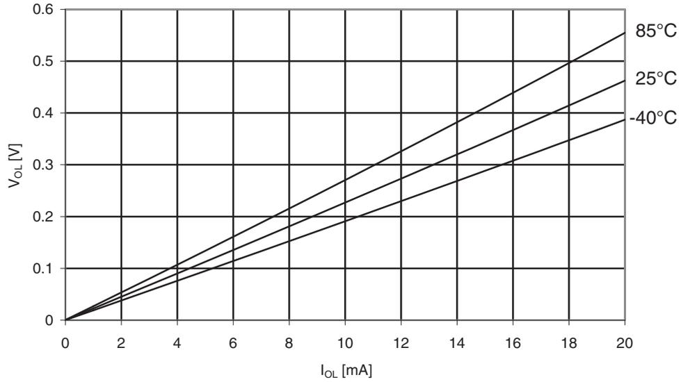
**Figure 30-368. ATmega1284P: I/O pin output voltage vs. source current ( $V_{CC} = 2.7V$ )**
