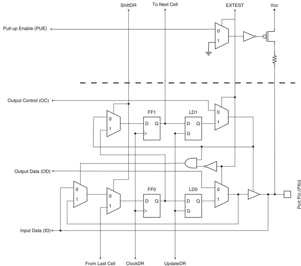
**Figure 25-4. General Port Pin schematic diagram**
