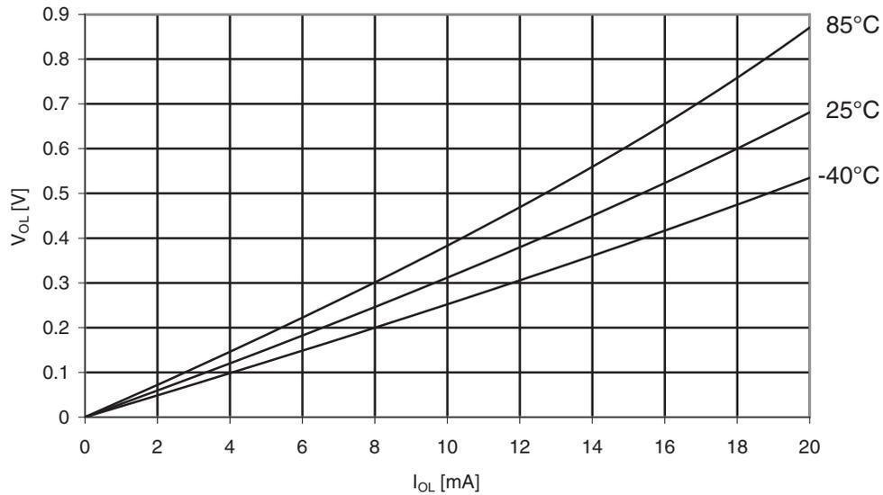
**Figure 30-367. ATmega1284P: I/O pin output voltage vs. sink current ( $V_{CC} = 5V$ )**
