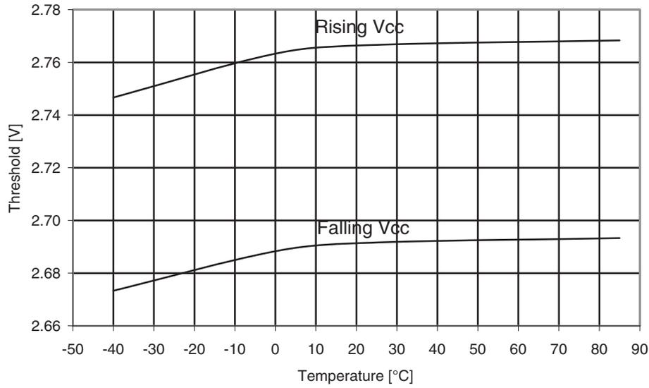
**Figure 30-378. ATmega1284P: BOD threshold vs. temperature ( $V_{BOT} = 1.8V$ )**
