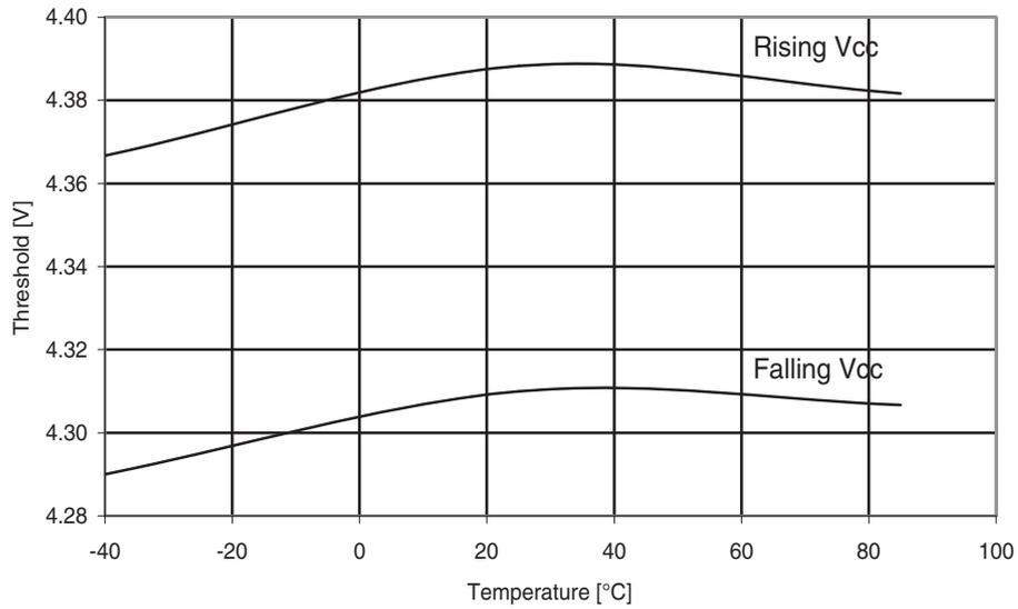
**Figure 30-179. ATmega324PA: BOD threshold vs. temperature ( $V_{BOT} = 2.7V$ ).**
