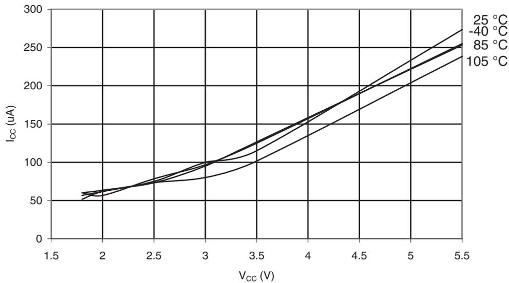
**Figure 31-75. Analog Comparator Current vs.  $V_{CC}$**
