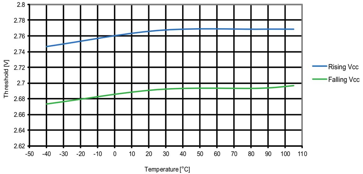
**Figure 31-148. ATmega1284P: BOD threshold vs. temperature ( $V_{BOT} = 1.8V$ )**
