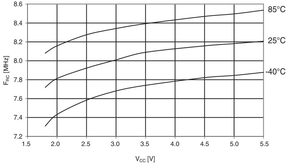
**Figure 30-334. ATmega1284: Calibrated 8MHz RC oscillator vs. temperature**
