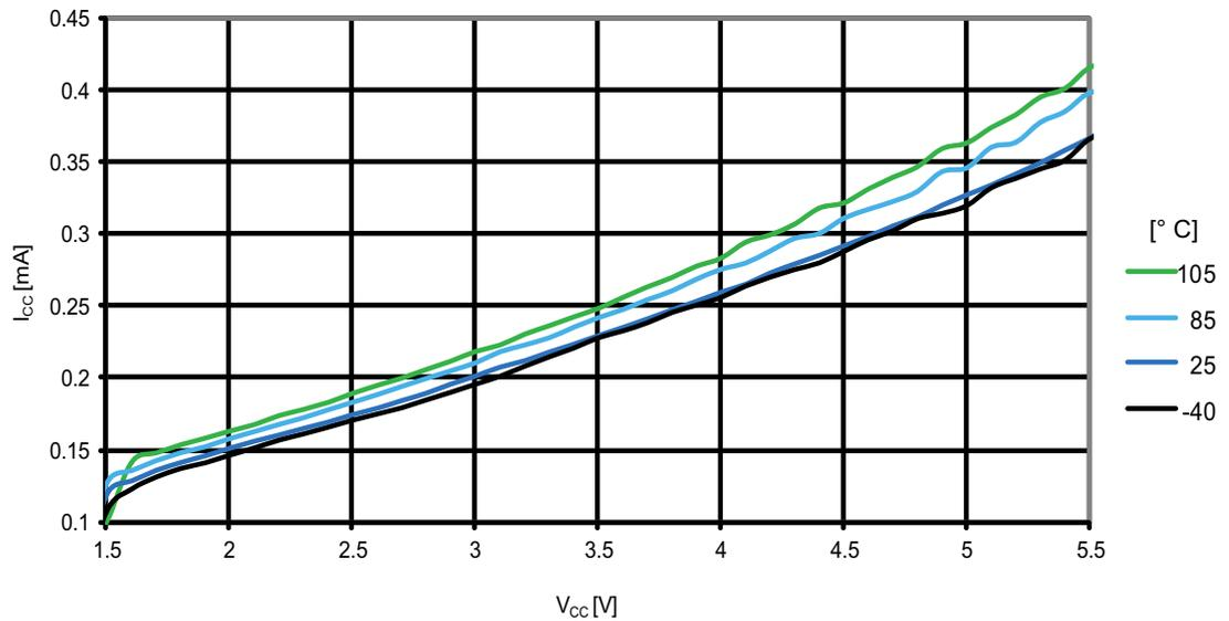
Figure 31-125. ATmega1284P: Idle supply current vs.  $V_{CC}$  (internal RC oscillator, 128kHz)
