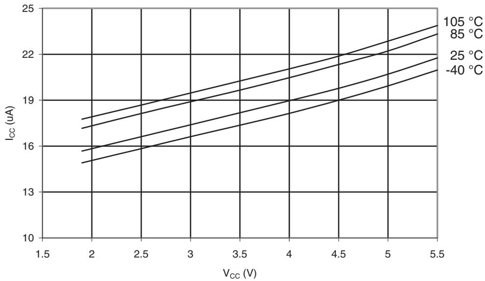
**Figure 31-117. Programming Current vs.  $V_{CC}$**
