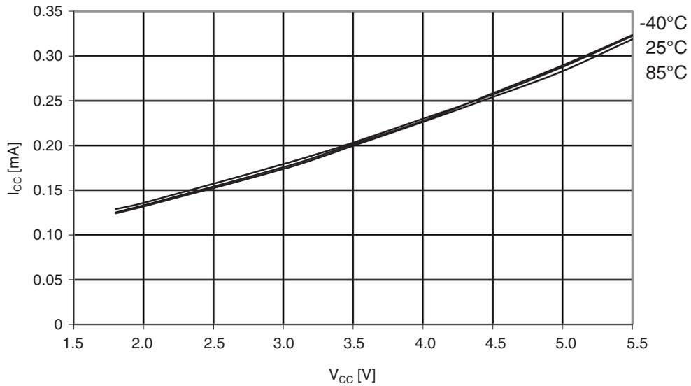
Figure 30-10. ATmega164A: Idle supply current vs.  $V_{CC}$  (internal RC oscillator, 128kHz)
