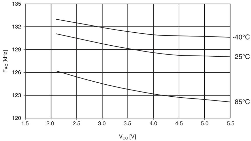
**Figure 30-87. ATmega164PA: Calibrated 8MHz RC oscillator vs.  $V_{CC}$**
