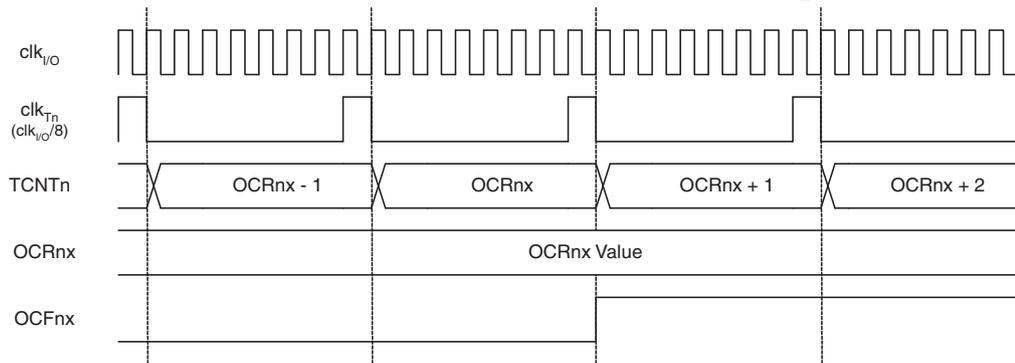
Figure 15-11 shows the setting of OCF0A and the clearing of TCNT0 in CTC mode and fast PWM mode where OCR0A is TOP.
