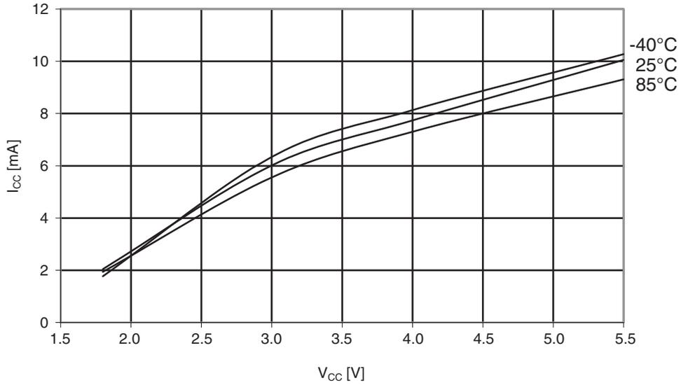
**Figure 30-95. ATmega164PA: Watchdog timer current vs.  $V_{CC}$**
