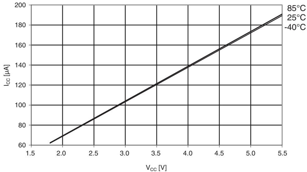
**Figure 30-339. ATmega1284: Brownout detector current vs.  $V_{CC}$**
