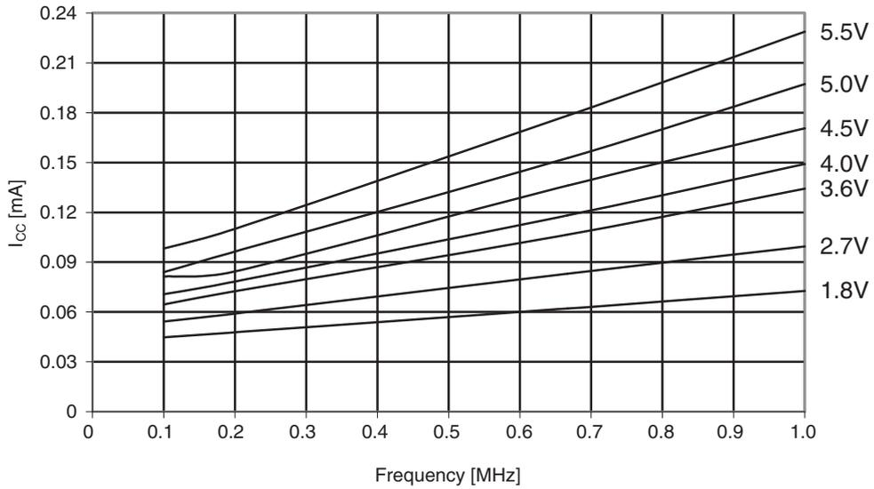
**Figure 30-301. ATmega1284: Idle supply current vs. frequency (1 - 20MHz)**
