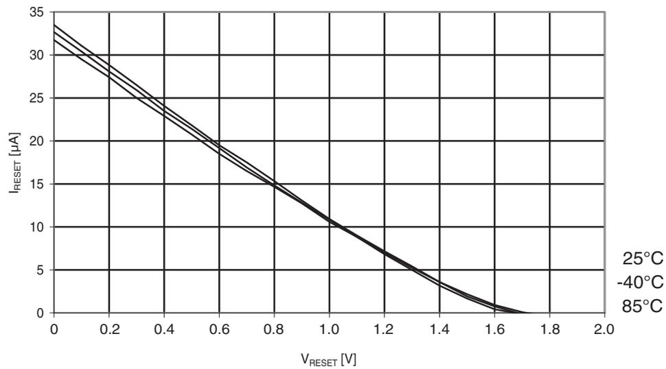
**Figure 30-264. ATmega644PA: Reset pull-up resistor current vs. reset pin voltage ( $V_{CC} = 2.7V$ )**
