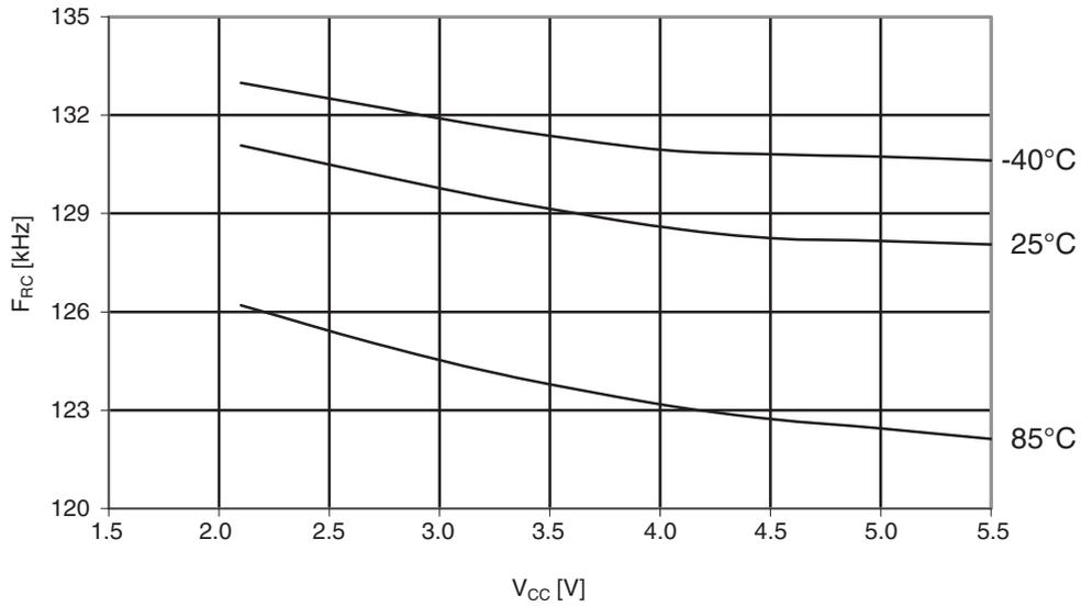
**Figure 30-38. ATmega164A: Calibrated 8MHz RC oscillator vs.  $V_{CC}$**
