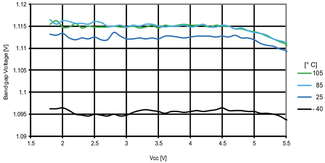
**Figure 31-150. ATmega1284P: Bandgap voltage vs. temperature**
