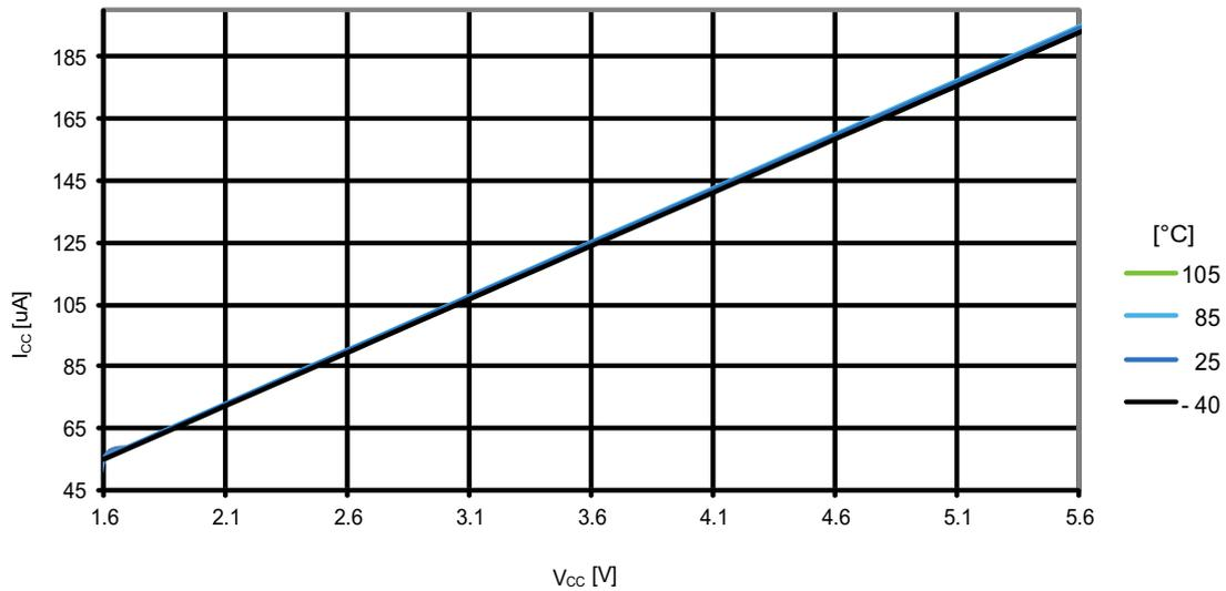
Figure 31-159. ATmega1284P: Brownout detector current vs.  $V_{CC}$
