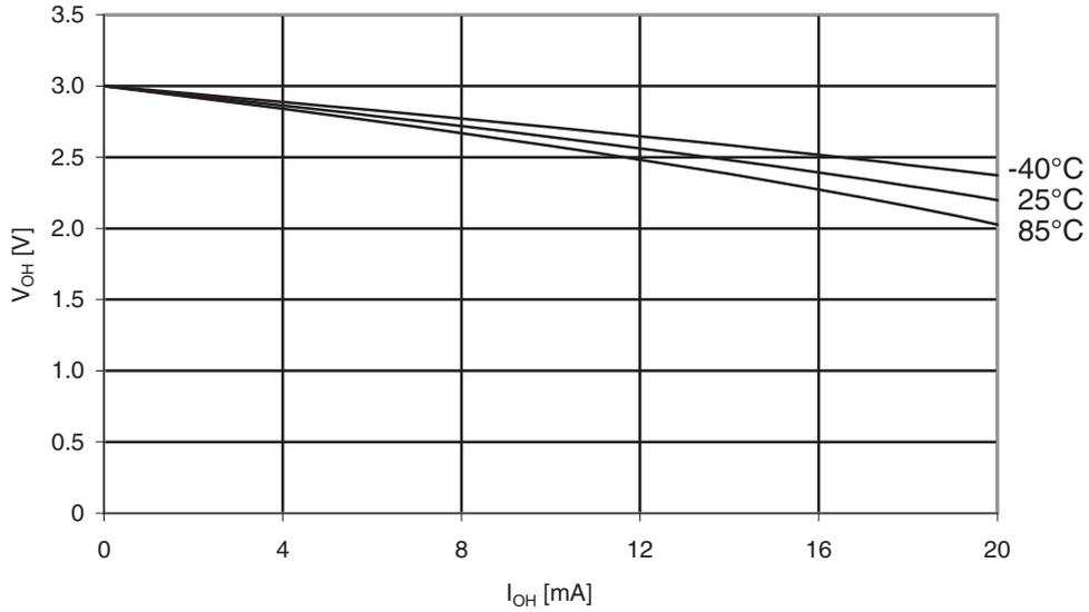
**Figure 30-73. ATmega164PA: I/O pin output voltage vs. source current ( $V_{CC} = 5V$ )**
