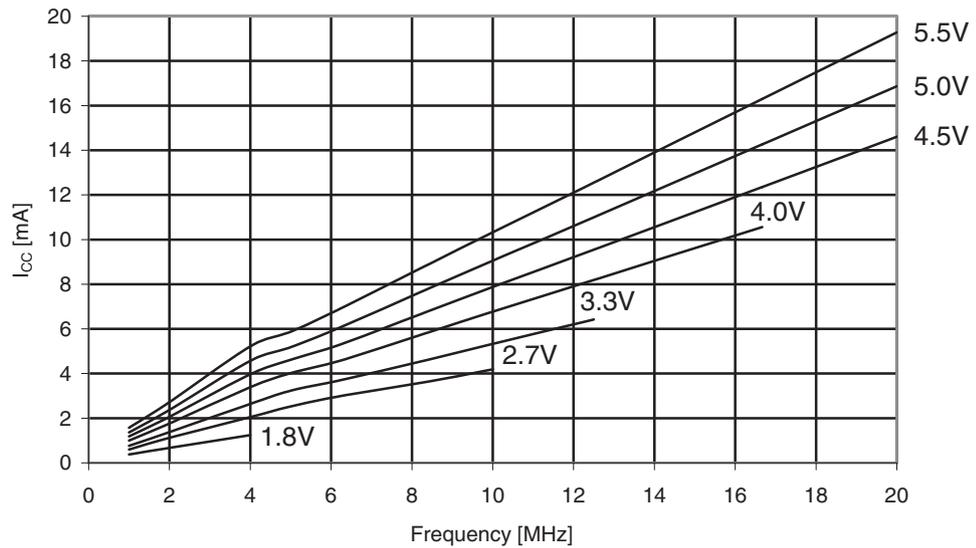
**Figure 30-347. ATmega1284P: Active supply current vs.  $V_{CC}$  (internal RC oscillator, 8MHz)**
