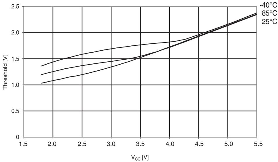
**Figure 30-127. ATmega324A: Reset pin input threshold vs.  $V_{CC}$  ( $V_{IL}$ , I/O pin read as '0')**
