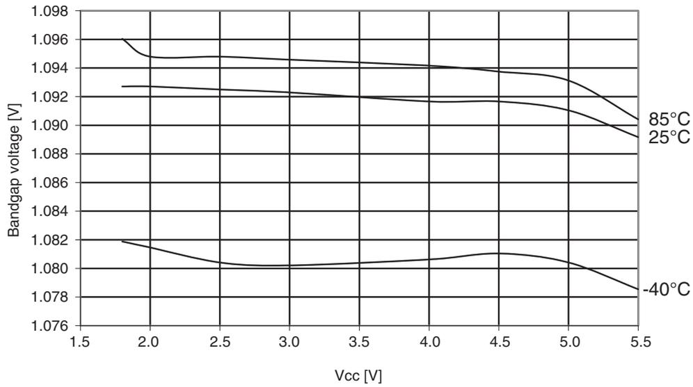
**Figure 30-182. ATmega324PA: Bandgap voltage vs. temperature**
