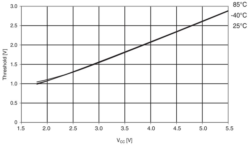
**Figure 30-124. ATmega324A: I/O pin input threshold vs.  $V_{CC}$  ( $V_{IL}$ , I/O pin read as '0')**
