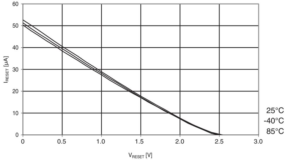
**Figure 30-216. ATmega644A: Reset pull-up resistor current vs. reset pin voltage ( $V_{CC} = 5V$ )**
