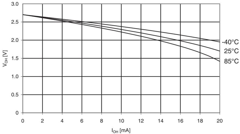
**Figure 30-369. ATmega1284P: I/O pin output voltage vs. source current ( $V_{CC} = 3V$ )**
