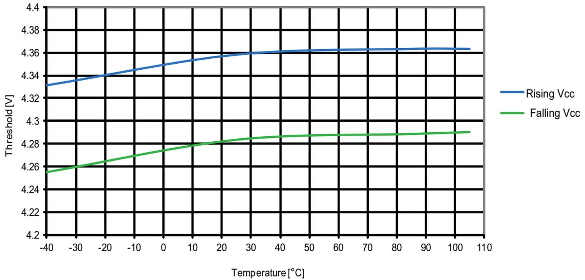
**Figure 31-147. ATmega1284P: BOD threshold vs. temperature ( $V_{BOT} = 2.7V$ )**
