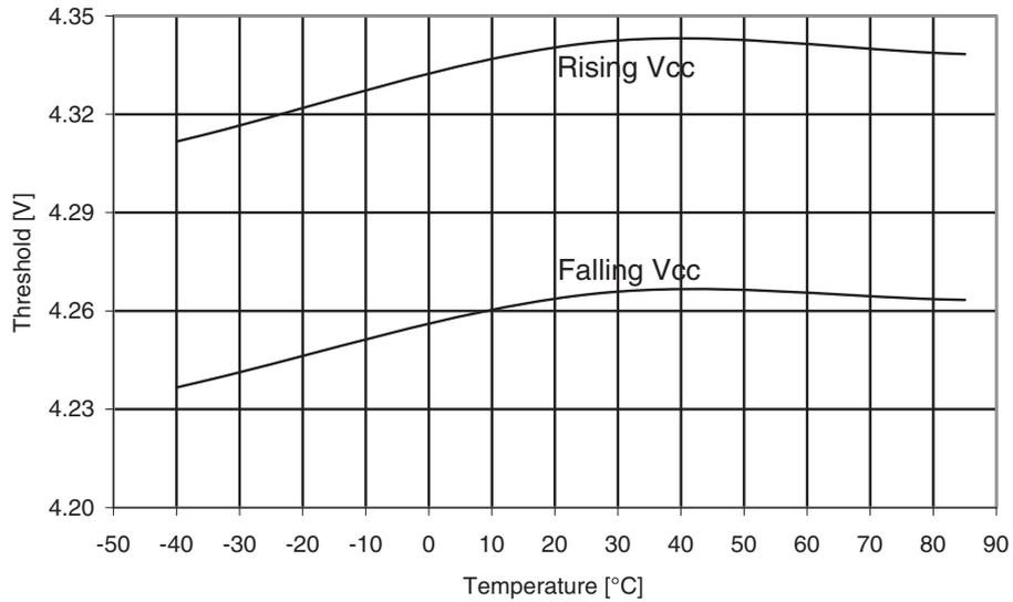
**Figure 30-277. ATmega644PA: BOD threshold vs. temperature ( $V_{BOT} = 2.7V$ )**
