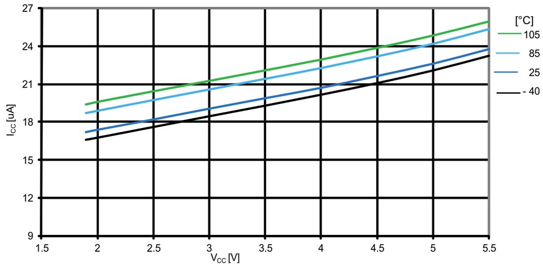
**Figure 31-39. ATmega164PA: Programming current vs.  $V_{CC}$**
