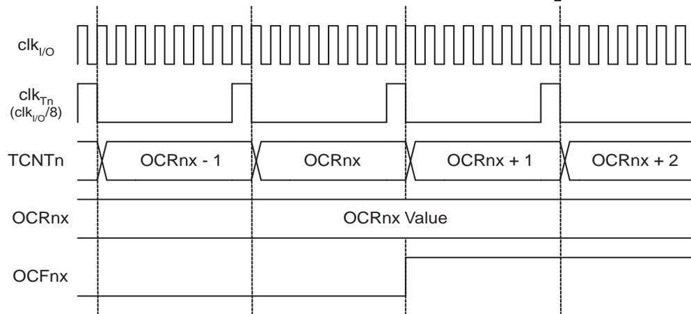
Figure 17-11 on page 156 shows the setting of OCF2A and the clearing of TCNT2 in CTC mode.
