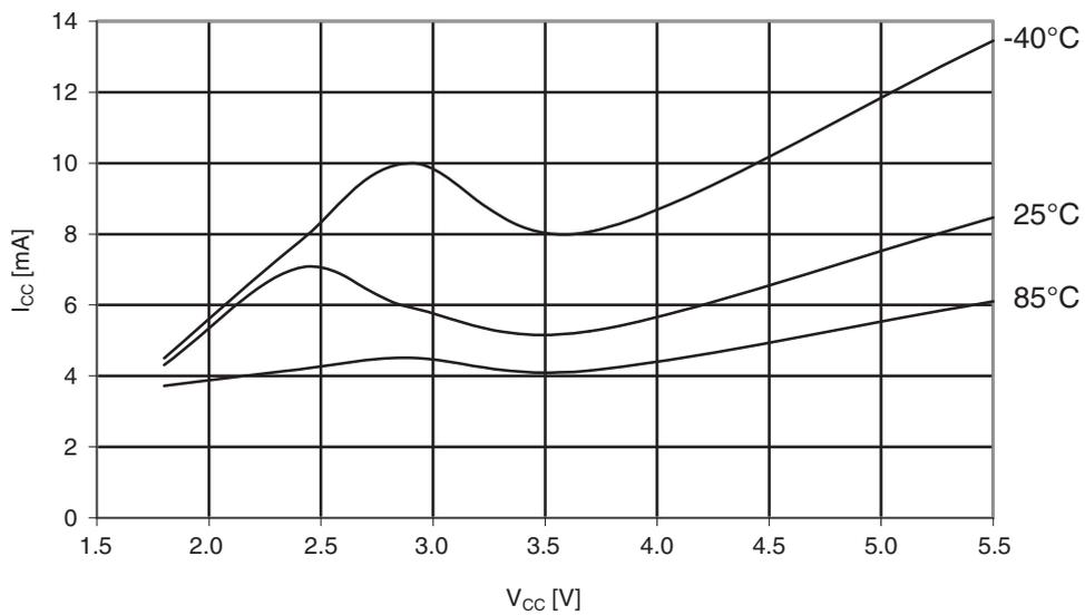
**Figure 30-391. ATmega1284P: Watchdog timer current vs.  $V_{CC}$**
