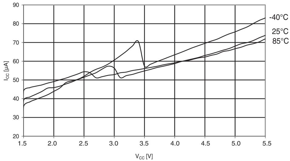
**Figure 30-239. ATmega644A: AREF external reference current vs.  $V_{CC}$**
