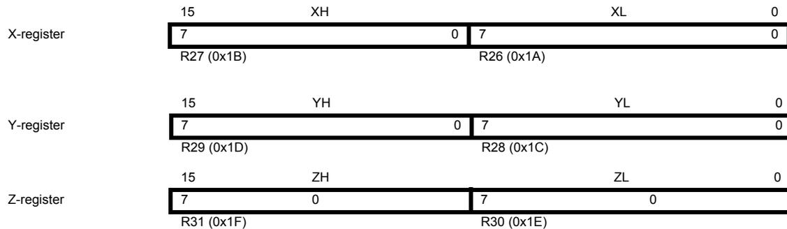
In the different addressing modes these address registers have functions as fixed displacement, automatic increment, and automatic decrement (see the AVR Instruction Set Manual for details).
