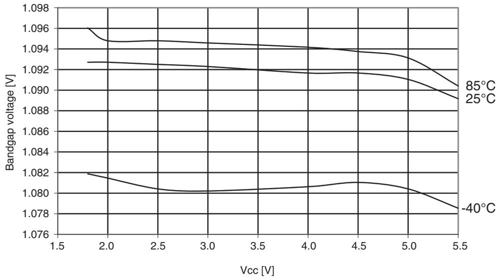
**Figure 30-133. ATmega324A: Bandgap voltage vs. temperature**
