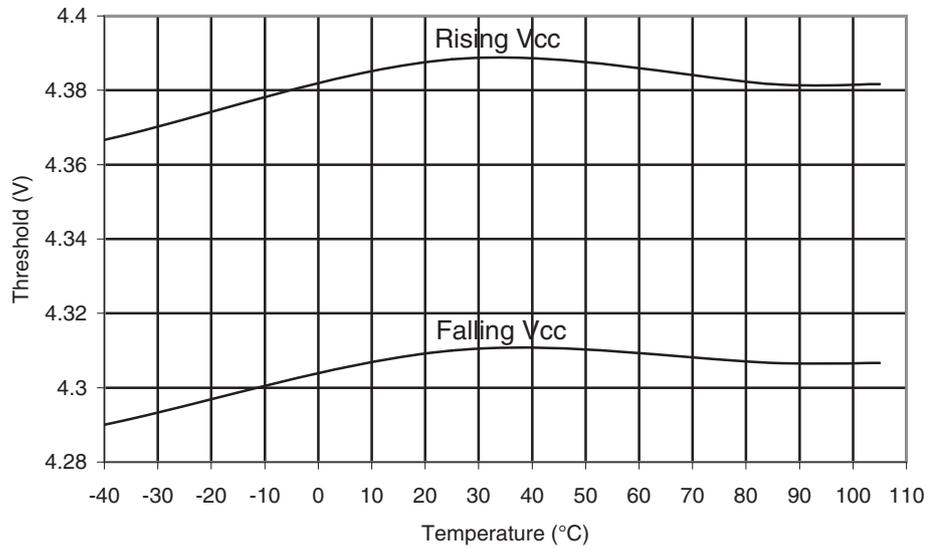
**Figure 31-67. BOD Threshold vs. Temperature ( $V_{CC} = 2.7V$ )**
