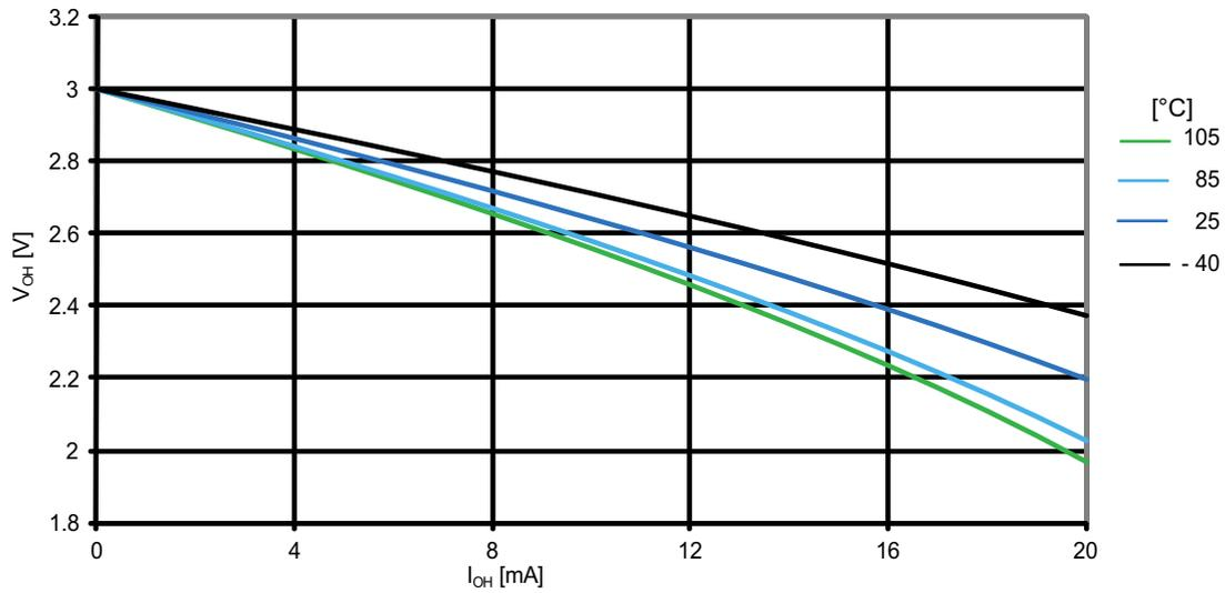
**Figure 31-18. ATmega164PA: I/O pin output voltage vs. source current ( $V_{CC} = 5V$ )**
