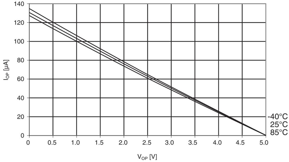
**Figure 30-362. ATmega1284P: Reset pull-up resistor current vs. reset pin voltage ( $V_{CC} = 1.8V$ )**
