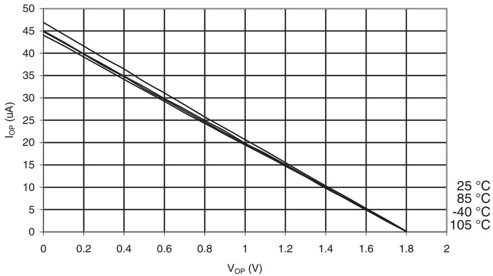
**Figure 31-51. I/O Pin Pull-up Resistor Current vs. Input Voltage ( $V_{CC} = 2.7V$ )**
