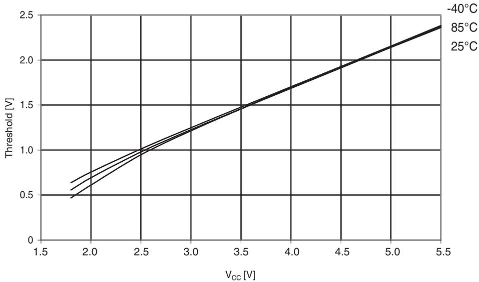
**Figure 30-125. ATmega324A: I/O pin input hysteresis vs.  $V_{CC}$**
