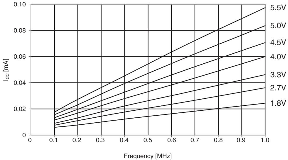
**Figure 30-343. ATmega1284: Reset supply current vs. frequency (1 - 20MHz)**
