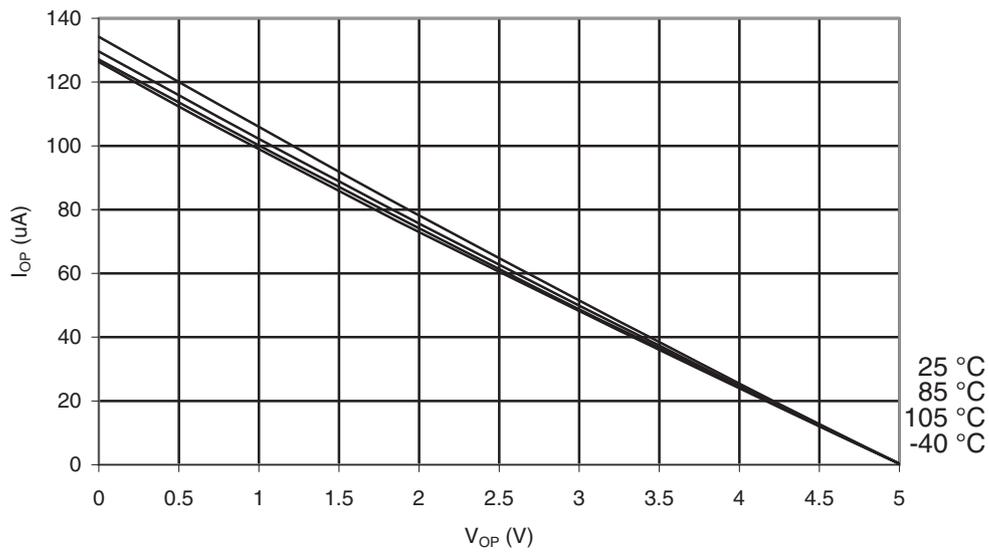
**Figure 31-53. Reset Pull-up Resistor Current vs. Reset Pin Voltage ( $V_{CC} = 1.8V$ )**
