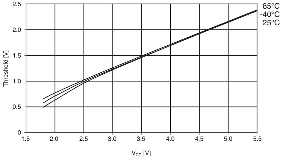
**Figure 30-372. ATmega1284P: I/O pin input hysteresis vs.  $V_{CC}$**
