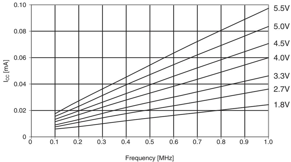
**Figure 30-393. ATmega1284P: Reset supply current vs. frequency (1 - 20MHz)**
