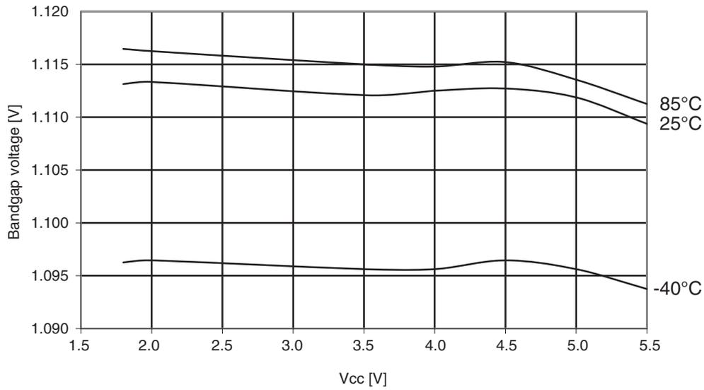
**Figure 30-330. ATmega1284: Bandgap voltage vs. temperature**
