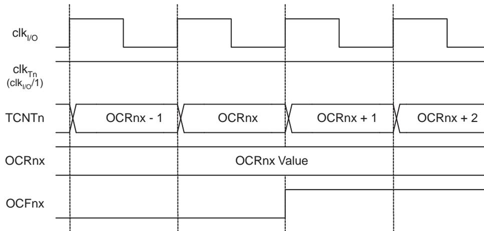
[Figure 16-11](#) shows the same timing data, but with the prescaler enabled.
