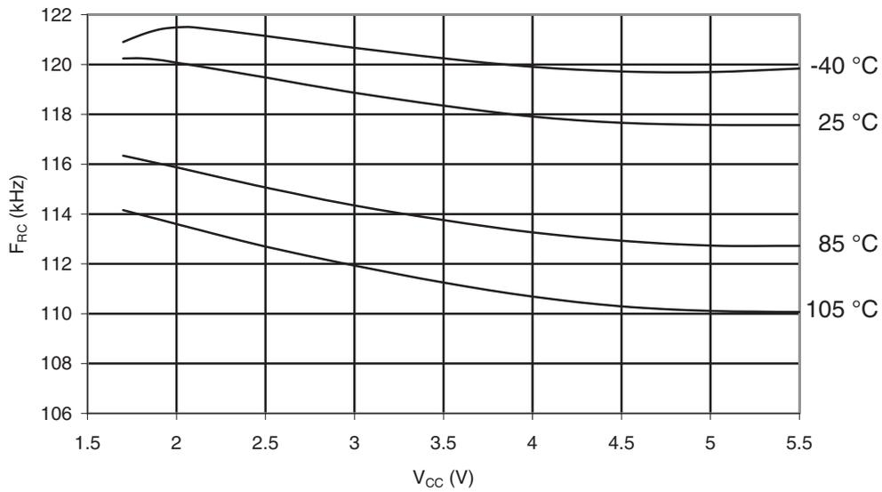
**Figure 31-71. Calibrated 8 MHz RC Oscillator vs.  $V_{CC}$**
