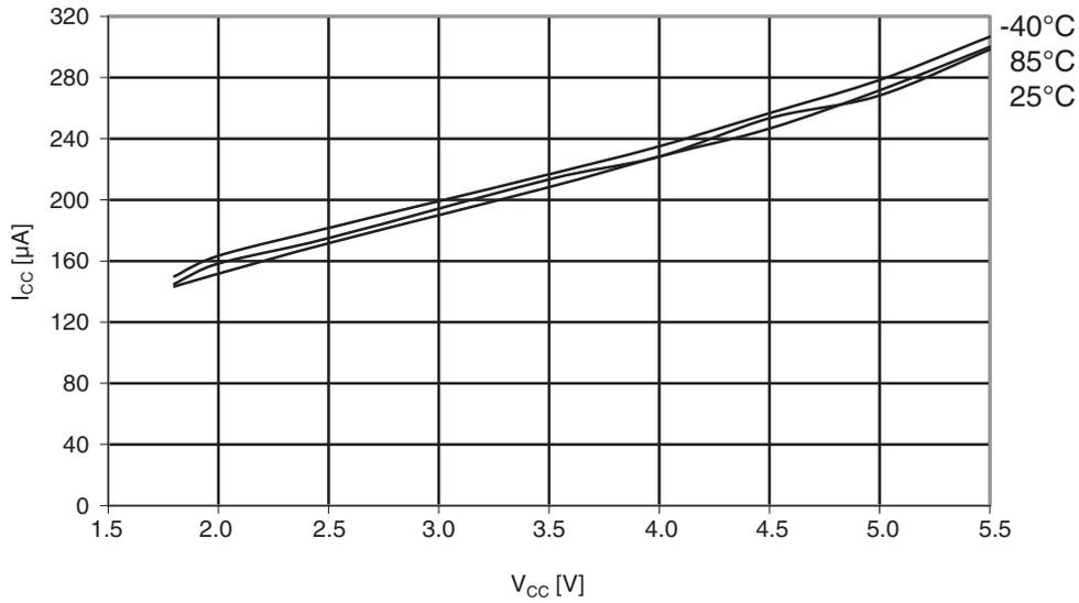
**Figure 30-91. ATmega164PA: Analog comparator current vs.  $V_{CC}$**
