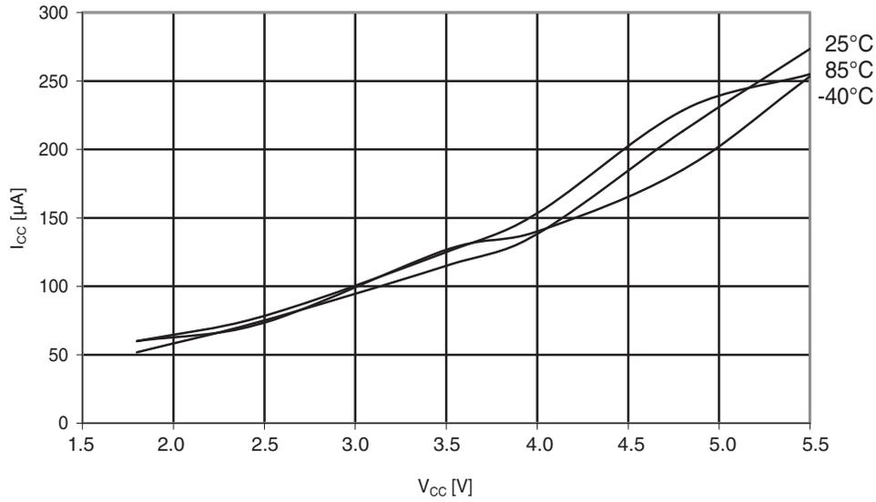
**Figure 30-140. ATmega324A: Analog comparator current vs.  $V_{CC}$**
