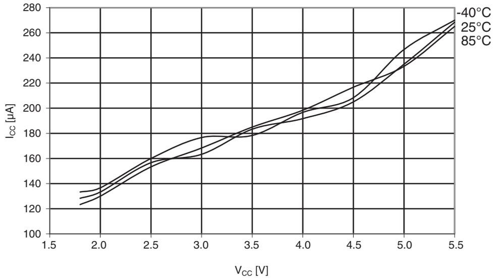
**Figure 30-337. ATmega1284: Analog comparator current vs.  $V_{CC}$**
