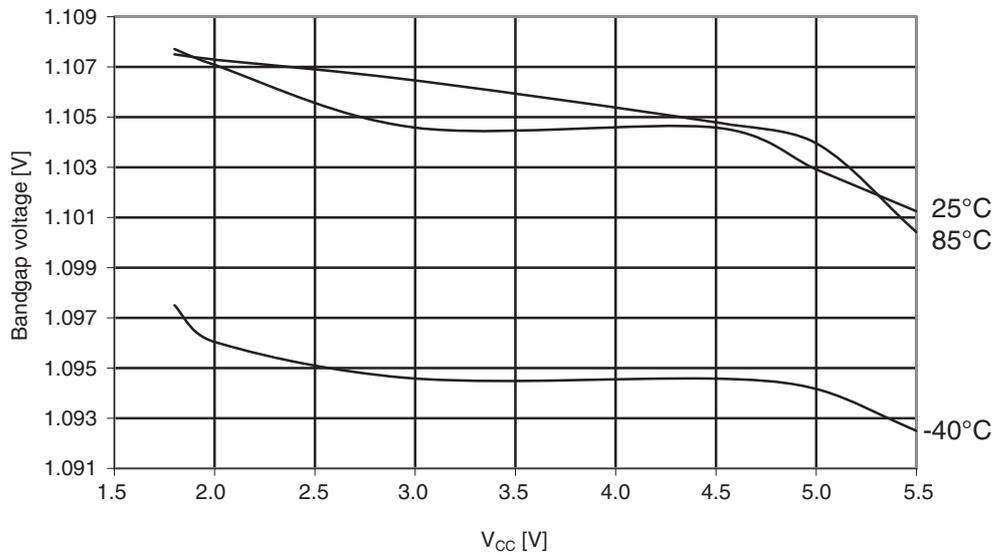
**Figure 30-35. ATmega164A: Bandgap voltage vs. temperature.**
