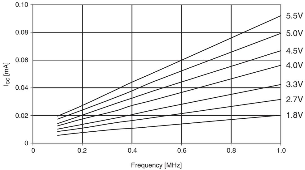
**Figure 30-97. ATmega164PA: Reset supply current vs. frequency (1 - 20MHz)**
