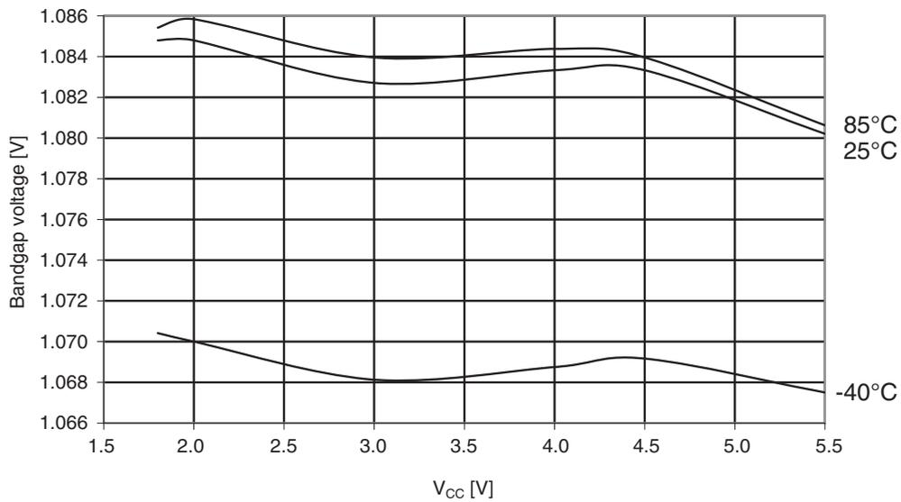
**Figure 30-280. ATmega324PA: Bandgap voltage vs. temperature**
