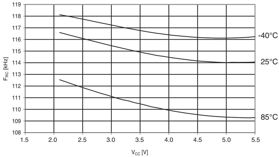
**Figure 30-283. ATmega644PA: Calibrated 8MHz RC oscillator vs.  $V_{CC}$**
