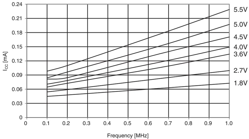
**Figure 30-351. ATmega1284P: Idle supply current vs. frequency (1 - 20MHz)**
