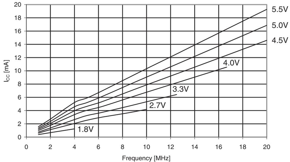
**Figure 30-297. ATmega1284: Active supply current vs.  $V_{CC}$  (internal RC oscillator, 8MHz)**
