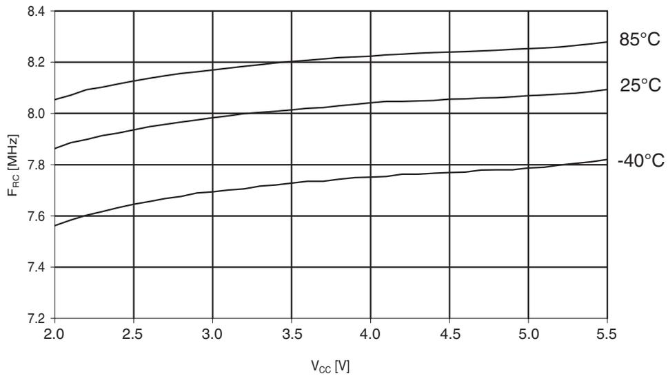
**Figure 30-284. ATmega644PA: Calibrated 8MHz RC oscillator vs. temperature**
