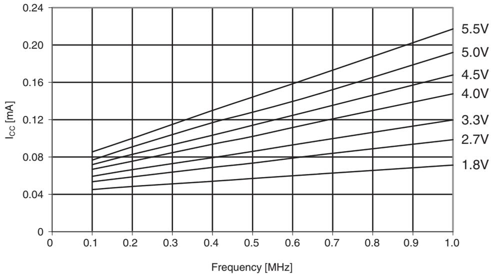
**Figure 30-203. ATmega644A: Idle supply current vs.  $V_{CC}$  (1 - 20MHz)**
