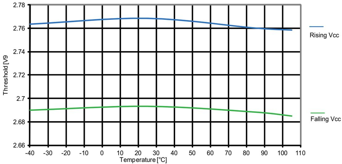
**Figure 31-27. ATmega164PA: BOD threshold vs. temperature ( $V_{BOT} = 1.8V$ )**
