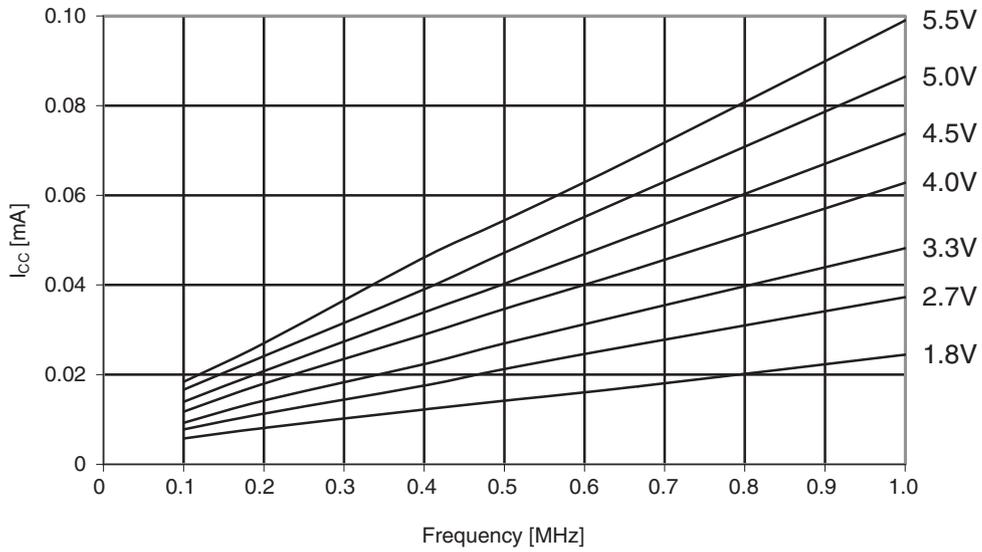
**Figure 30-244. ATmega644A: Reset supply current vs. frequency (1 - 20MHz)**
