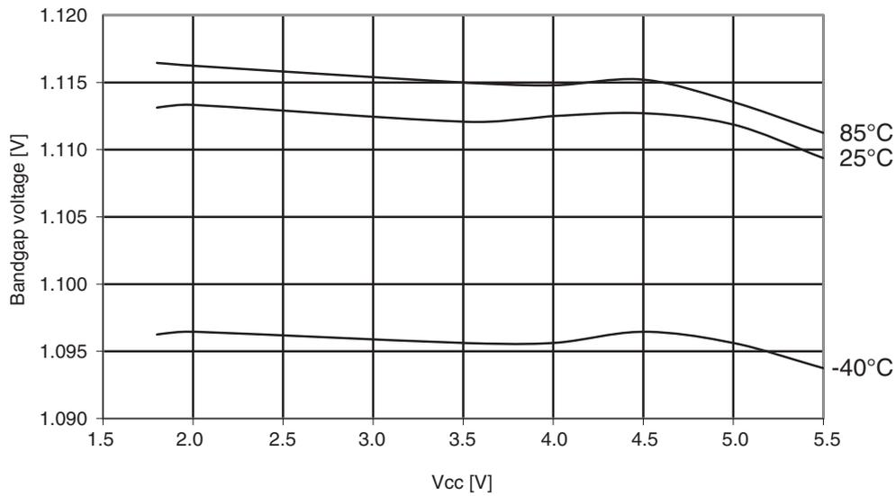
**Figure 30-380. ATmega1284P: Bandgap voltage vs. temperature**
