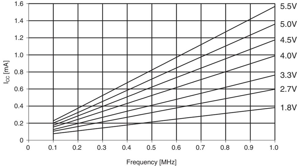
Figure 30-296. ATmega1284: Active supply current vs. frequency (1 - 20MHz)
