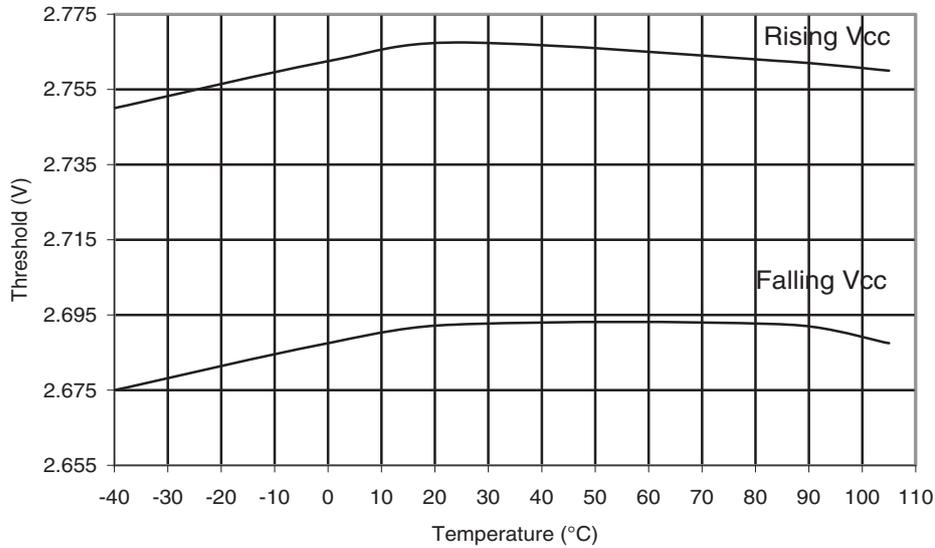
**Figure 31-107. BOD Threshold vs. Temperature ( $V_{CC} = 1.8V$ )**
