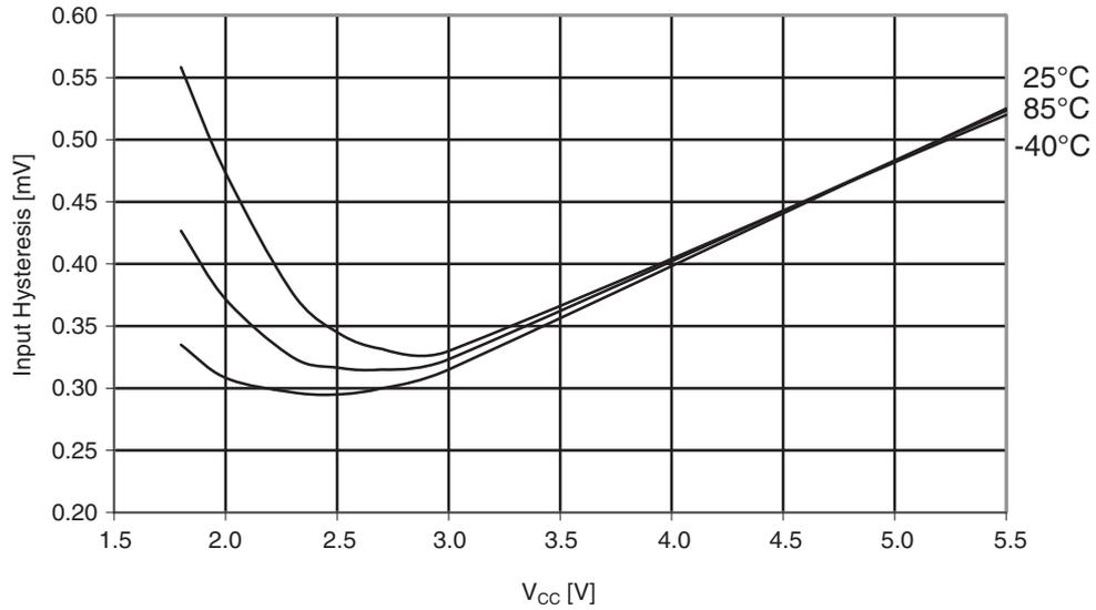
**Figure 30-224. ATmega644A: Reset pin input threshold vs.  $V_{CC}$  ( $V_{IH}$ , I/O pin read as '1')**
