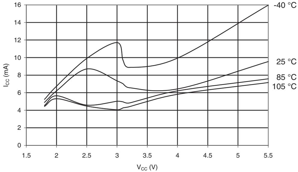
**Figure 31-118. Watchdog Timer Current vs.  $V_{CC}$**
