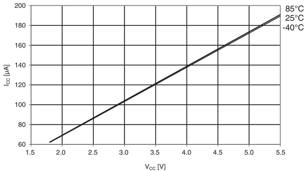
**Figure 30-389. ATmega1284P: Brownout detector current vs.  $V_{CC}$**
