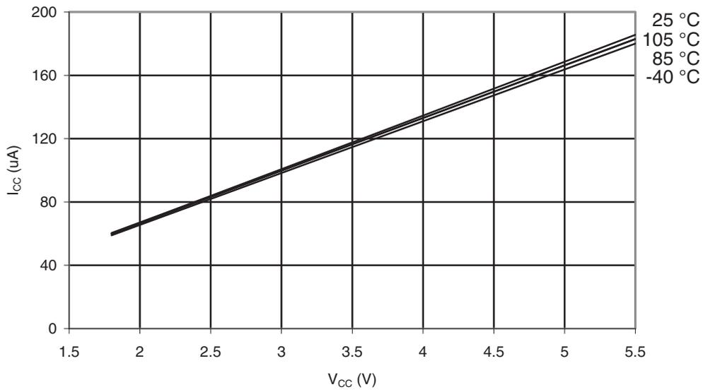
**Figure 31-77. Brownout Detector Current vs.  $V_{CC}$**
