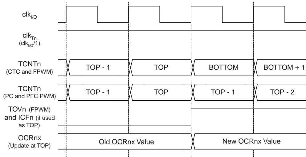
Figure 16-13 shows the same timing data, but with the prescaler enabled.
