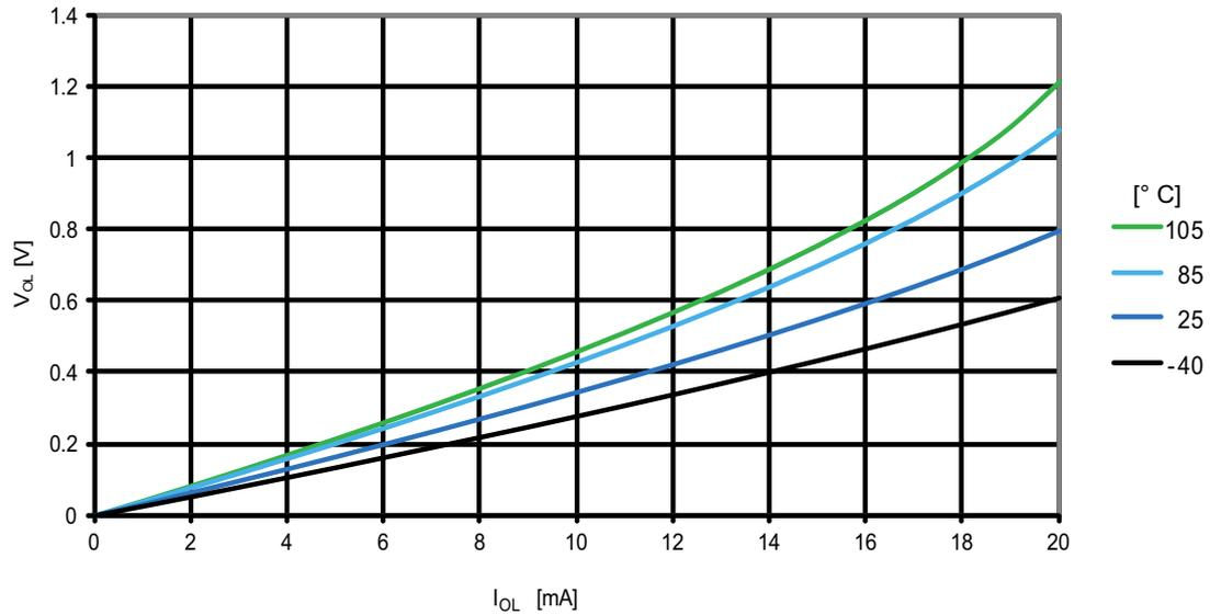
Figure 31-136. ATmega1284P: I/O pin output voltage vs. sink current ( $V_{CC} = 3V$ )
