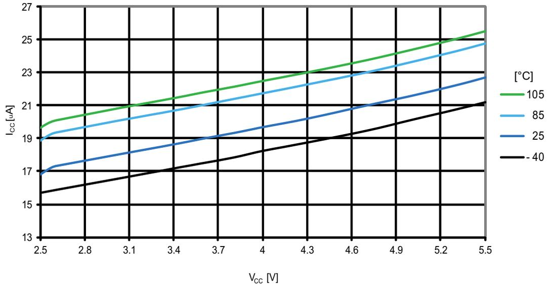
Figure 31-160. ATmega1284P: Programming current vs.  $V_{CC}$
