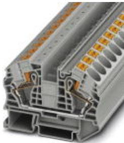
Feed-through terminal block, Connection method: Push-in connection, Cross section: 0.5 mm 2 - 25 mm 2 , AWG: 20 - 4, Width: 12.2 mm, Color: black, Mounting type: NS 35/7,5, NS 35/15
