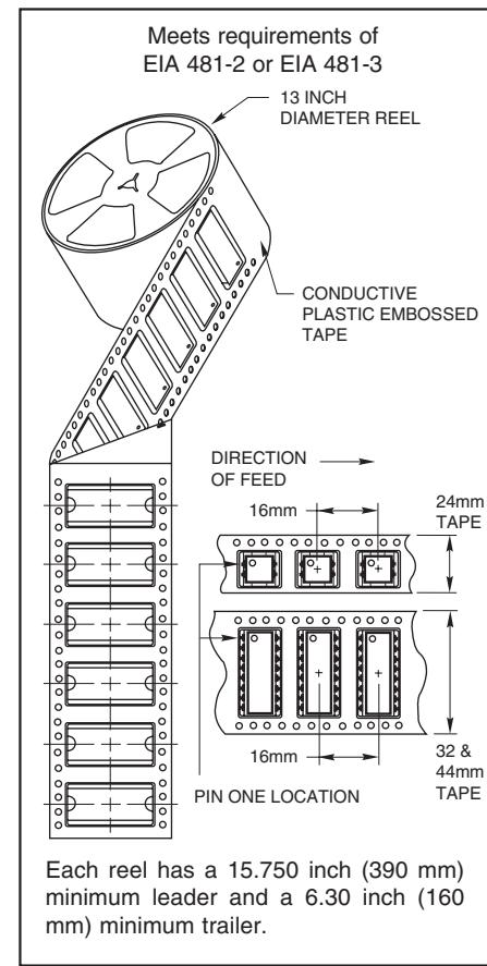
Each reel has a 15.750 inch (390 mm) minimum leader and a 6.30 inch (160 mm) minimum trailer.
