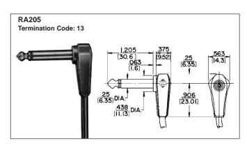
**RA200:** Right-angle phone plug with plastic handle. Body extension suitable for recessed jack. Completely shielded.
