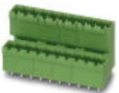
Header, Nominal current: 10 A, Rated voltage (III/2): 320 V, Number of positions: 8, Pitch: 5.08 mm, Color: green, Contact surface: Tin, Assembly: Soldering, The article can be aligned to create different nos. of positions! In combination with MVSTB or FKCV plug components, both an MVSTBW (or FKCVW) and an MVSTBR plug (or FKCVR) must be used. Combination with TMSTBP plug components is not possible!
