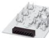
Header, Nominal current: 12 A, Rated voltage (III/2): 320 V, Number of positions: 8, Pitch: 5.08 mm, Color: black, Contact surface: Tin, Assembly: SMD/THT/THR, User information and design recommendations for through hole reflow technology can be found under "Downloads"
