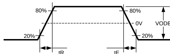
Figure 1. Driver Output Transition Time
