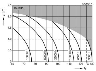
**Useful life**<sup>1)</sup> depending on ambient temperature  $T_A$  under ripple current operating conditions I > 25 mm
