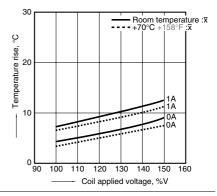
5-(2). Coil temperature rise Tested sample: TXS2-24V, 6 pcs. Point measured: Inside the coil Ambient temperature: 25°C 77°F, 70°C 158°F
