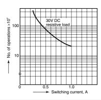
3. Mechanical life Tested sample: TXS2-4.5V, 10 pcs. Operating speed: 180 cpm
