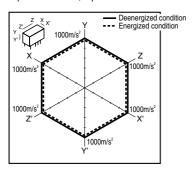
9-(2). Malfunctional shock (latching) Tested sample: TXS2-L2-4.5V, 6 pcs.
